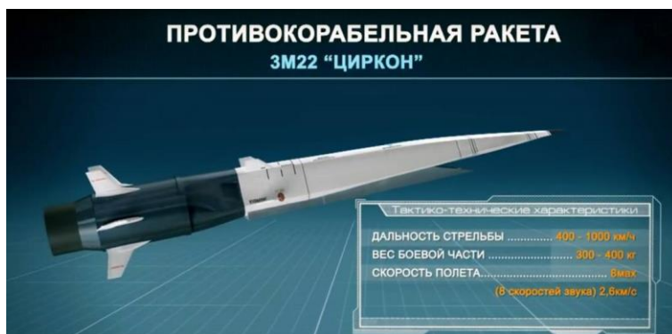
Figure 1: Basic data of the anti-ship hypersonic missile “Zircon.”
