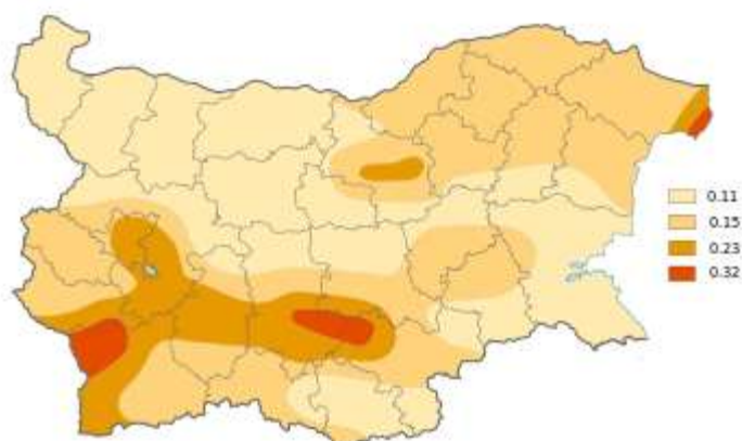
Figure 6: Map of seismic hazards showing maximum values of acceleration of the ground in (g) with a period of repeatability 475 years.
